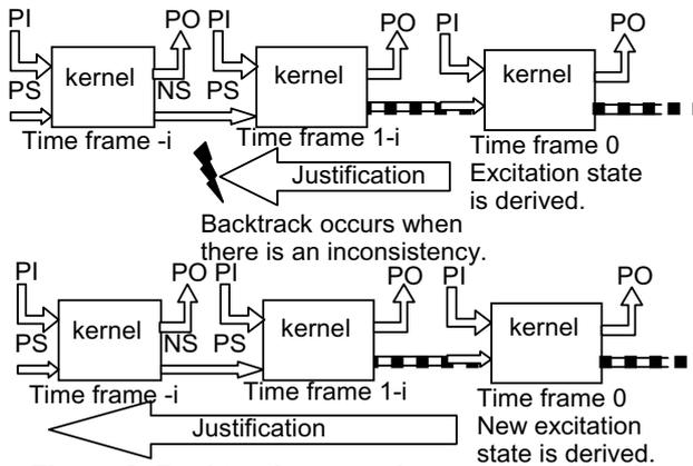
**Figure 3. Backtrack occurs between justification and derivation of excitation state.**
