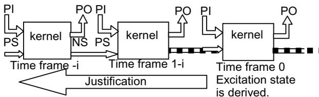
**Figure 4. No backtrack between justification and derivation of excitation state.**
