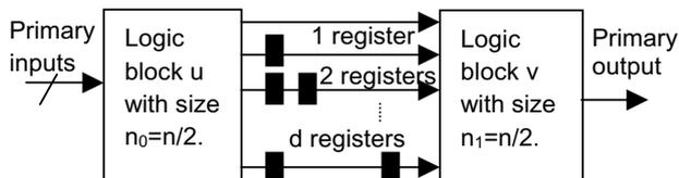
Figure 1. Block diagram of the structure of C.
