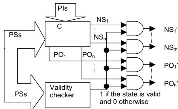
**Figure 5. Transformed combinational part C' embedded with a validity checker.**
