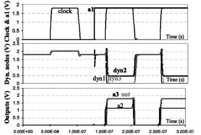
Figure 8: Time diagrams of the voltage levels, GOS in Na (1 node centered, 1\Omega , 10MHz)
