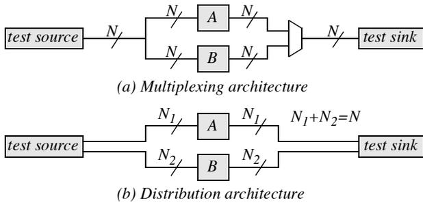
**Figure 7. Multiplexing architecture and distribution architecture [1].**
