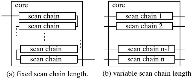
Figure 2. Scan-chains design at a core.
