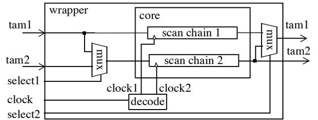
Figure 3. Flexible power conscious scan-chains design at a core test wrapper.
