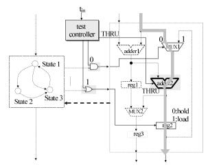
Figure 8. Test architecture of the proposed method
