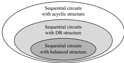
**Figure 6. Classification of sequential circuits by structure.**
