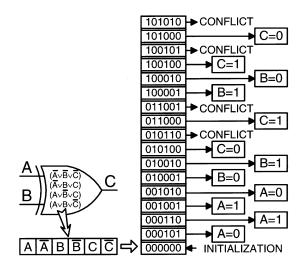
Fig. 5. Representation of direct A-implications for two-input XOR gate.
