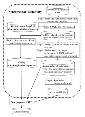
Fig. 4 The flow chart of the proposed method.
