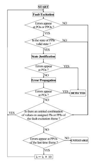
**Fig.7** The flow chart of the proposed test generation method for sequential circuits.
