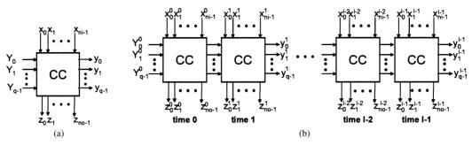
Fig. 3 A time frame of a sequential circuit  $M_s$  (a) and a time frame expansion model of  $M_s$  (b).
