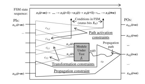
**Fig. 3** An unrolled RTL circuit with test generation constraints for a test path for a MUT
