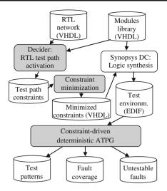
Fig. 1 Constraint-based untestability proof flow
