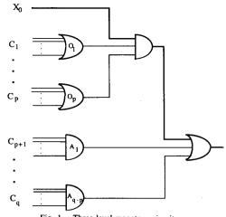
Fig. 1. Three-level monotone circuits.
