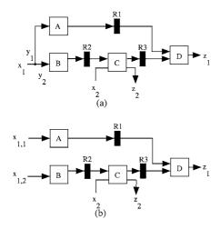
*Fig.* 4. (a) Example of internally balanced structure, (b) Circuit resulting from the operation (1) of the C\*-transformation.
