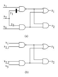
*Fig. 5.* (a) Internally balanced structure *S*, (b) Combinational equivalent  $C^*(S)$ .
