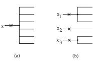
*Fig. 1.* Correspondence of faults: (a) A separable primary input in *S*, (b) separated primary inputs in *C*.
